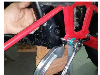
Insert a **thin** 303 SS spacer into each side of the ball on the outside end heim joint. Bring the radius arm up and carefully slide the heim spacers into the opening in the carrier. Insert the OEM Bolt Loctite and install the OEM nut. Tighten to 50 ft. lbs.
