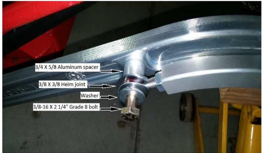
Add 3/8" jam nut with Loctite on back side of radius arm and tighten.
