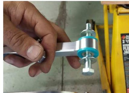
Position the inside heim between the frame and the back plate so all of the holes line up. Insert the 10 mm bolt with the control arm and washers through the back plate, spacers and frame as shown. Install lock nut with Loctite. Hold the nut in place with a 17MM wrench from back side. Tighten bolt to 50 ft. lbs.
