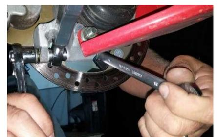
7. Thread the 3/8 X 3/8" heim joint with jam nut into the end of the control arm. Do not tighten jam nut yet. Adjust length of heim so the 3/8 hole lines up straight with the threaded hole in the radius arm.
