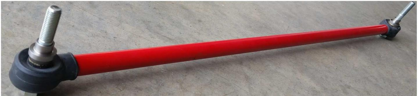
5. Use the stock radius arm to set length by placing two of the long 10 MM bolts through the ball joints. Lay the stock arm on a flat surface so the bolts are standing straight up as shown. Place one of the 303 SS spacers over each bolt with the small diameter facing up.
