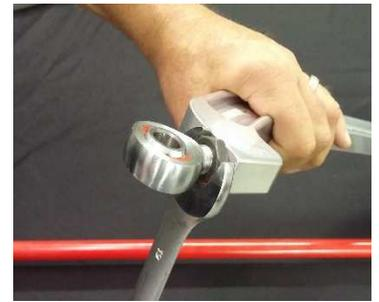
6. Insert a **thick** 303 SS spacer into each side of the ball on the inside end heim joint and set aside. Place the 10 X 80 MM grade 8 bolt through a washer then through the spacer/bushing of the control arm and then through another washer.
