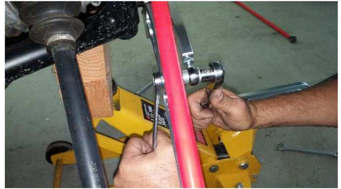
Hold the control arm in place with a 5/8" open end wrench and tighten the jam nut on the 3/8" heim with a 9/16" open end wrench. Repeat the entire operation for the opposite side. Replace wheels, remove jack stands and you're done!
